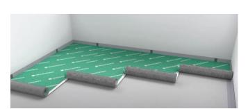
Install the acoustic mat with rubber granules facing down
