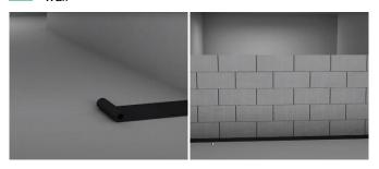
Apply in the first wall a layer of row mortar of about 1 cm thickness
