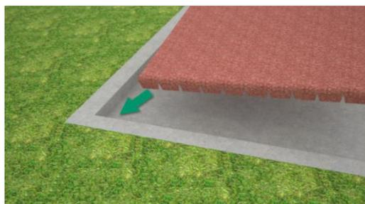
Start the installation from the corner of the surface to be covered leaving exposed the pad side prepared for the connectors.
