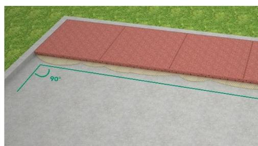
Install the first row of tiles to the edge of the other side taking care for a proper alignment and perpendicularity
