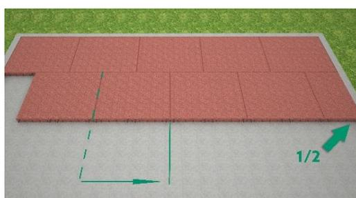
Install the second row offsetting to the first row of half plate. Continue offsetting the other rows to complete the surface
