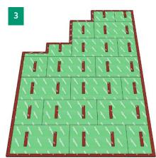
The sand and cement screed or leveling screed must have a thickness of more than 6 cm and a density of at least 2000 kg / m³ and must also be reinforced by a reinforcement mesh of 5 mm diameter and 200 mm mesh positioned at a height of about 20 mm from the top of the resilient mattress. For screed thicknesses greater than 100 mm, use a wooden panel as a disposable formwork (at least 15 mm thick) [4]. Before casting, protect the surface with a waterproof sheet.
