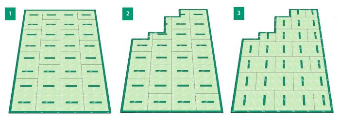
The sand and cement screed or leveling screed must have a thickness of more than 6 cm and a density of at least 2000 kg / m³ and must also be reinforced by a reinforcement mesh of 5 mm diameter and 200 mm mesh positioned at a height of about 20 mm from the top of the resilient mattress. For screed thicknesses greater than 100 mm, use a wooden panel as a disposable formwork (at least 15 mm thick) [4]. Before casting, protect the surface with a waterproof sheet.
