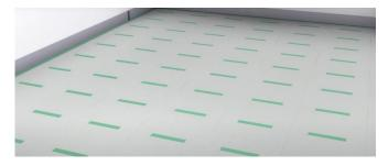
Apply a waterproof foil on the whole surface to protect the resilient layer.
