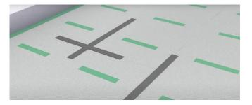
Install the reinforcement mesh (Ø 5 mm, net 200 mm) and build the screed (th. > 60 mm).
