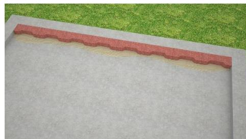
Start the second row with a tile of "Interlocking Cut O"
