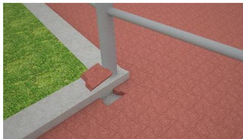
Cut tiles in a proper size and insert them in the blanks: use the special pieces "Cut V" or "Cut O" when possible
