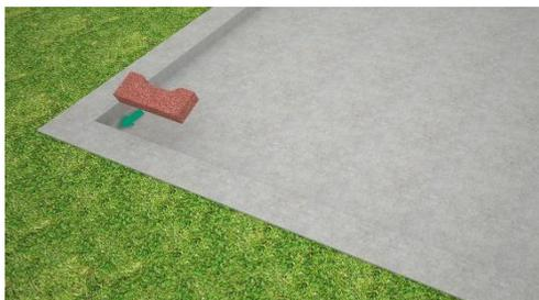
Start the installation from a corner of the tile surface with a "Interlocking cut V"
