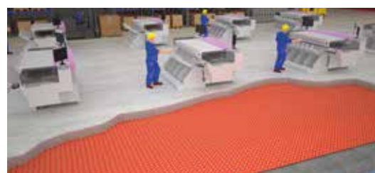
Isolation of textile production plant. MEGAPOINT line
